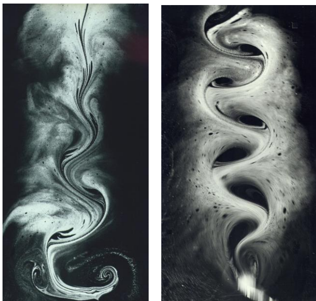
Kármán vortex paths indicating forms found in nature (Based on the work of T. Schwenk and J. Wilkes)
